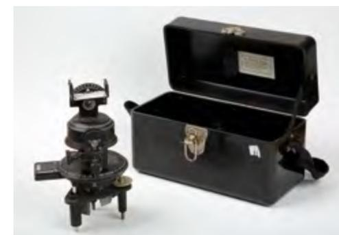
Astrocompass used by the navigators of British bomber planes
