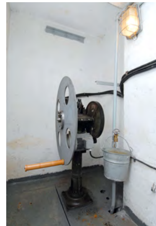
The "Royal" pump, performance 21 litres per minute, can pump water from depths of up to 150 metres
