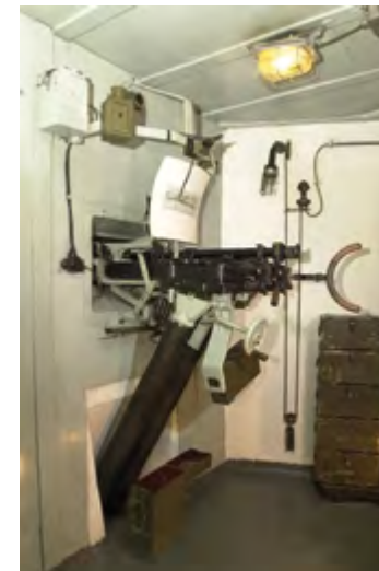
Pair of type-37, 7.92 mm heavy machine-guns in right-hand gun position of MO-S 19 Alej
